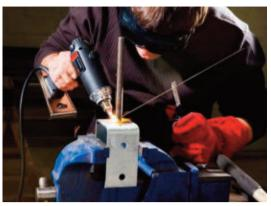
The Multiplaz 3500 power source can be used for welding and cutting jobs and requires no gases for either application. It requires only a tailored 8-oz. mixture of alcohol and water to help generate a plasma flame for welding and requires only 8 oz. of water to generate a cutting flame.
