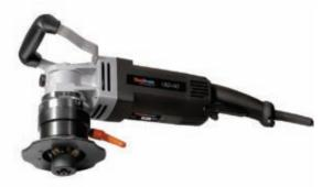
Variable electronic speed control allows adjustment of RPM to perform bevels on many types of material. Radius inserts uniformly break sharp edges for paint and coating preparation.
