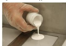
geometries in electronic applications. It can also be used for adhering integrated circuit substrates, base plates or heat sinks, or where grooves require a limited flow material. The liquid can be loaded into syringes and dispensed as a one-part material in bond lines as thin as 5 microns. Its adhesive strength can be improved with a primer.
