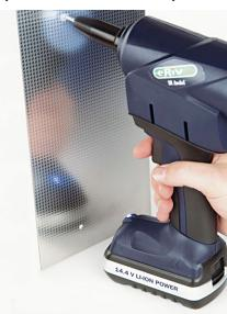
21-millimeter-long stroke that can place breakstem rivets with a nominal diameter of 3 to 5 millimeters. The tool has a pull force of 9 kilonewtons and a 2-second cycle time. Battery charge time is 1 hour.
