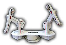
mounted to a programmable carousel. The robots' K11R controllers are interconnected, enabling communications to synchronize the motions of the robots moving together, or allowing the robots to cooperatively alternate turns while performing one task. Including the carousel, the system has a total of 11 axes. It also includes RoboForth II software, intuitive teach pad, cables and simple interfacing with other equipment.
