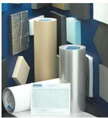
and urethane foam frequently used by manufacturers in the automotive, medical device, electronics and transportation markets. Series 654T-74-54 is a thin, lightweight tissue coated on both sides with 2 mils of high-tack, high-shear acrylic. Series 653-74-54 is a 3-mil acrylic film cast on a silicone-coated release liner. Series 654M-74-54 has 2 mils of acrylic on both sides of a high-quality polyester film.
