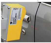
percent noncontact product inspection at scan rates up to 32 kilohertz. Each sensor uses a precalibrated laser, camera and optics to deliver consistent, reliable and precise real-world measurements. The sensor produces high-resolution images at distances up to 2 meters. It fits in small spaces and integrates without costly system modifications. The interface allows users to setup and control the sensor from a Web browser.
