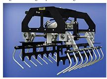
290 to 450 millimeters wide. The tooling weighs 17 kilograms and features 16 stainless steel fingers designed to withstand harsh manufacturing environments. Its main frame is made of lightweight aluminum. Spring-return decking plates ensure accurate placement of each bag onto a pallet. Other features include highflow pneumatic solenoid valves and a bag presence sensor.
