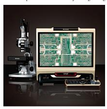
advanced zoom optics with a CCD camera, the microscope streamlines testing and improves inspection speed. It has a magnification range from 0.1 to 5,000 times and comes with a 17-inch LCD monitor, light source, controller and analysis-reporting software. The microscope can be equipped with a motorized XY stage and Z-axis lens control.
