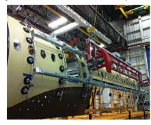
horizontal or pitched (up to 180 degrees) pieces that weigh thousands of pounds. The pieces can be smooth, rough or porous; made of sheet metal, glass or wood; and be of various shapes, including coils, sheets, planks, beams, barrels or drums. Recently, the company made a custom system for a commercial aircraft OEM to lift, rotate and reposition five separate fuselage panels.
